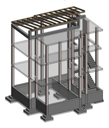
Model of reinforcing skeleton of reinforced concrete frame construction:
