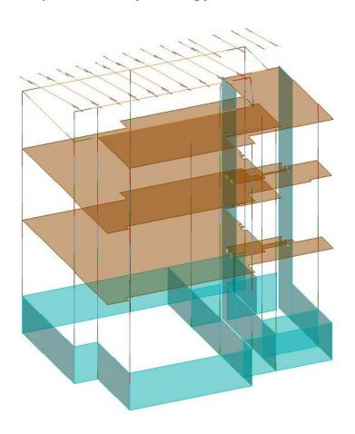
Analytical model of building frame in Autodesk Robot structural analysis:
